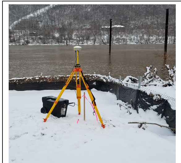
Figure 2.1 – Typical Base Station Setup
