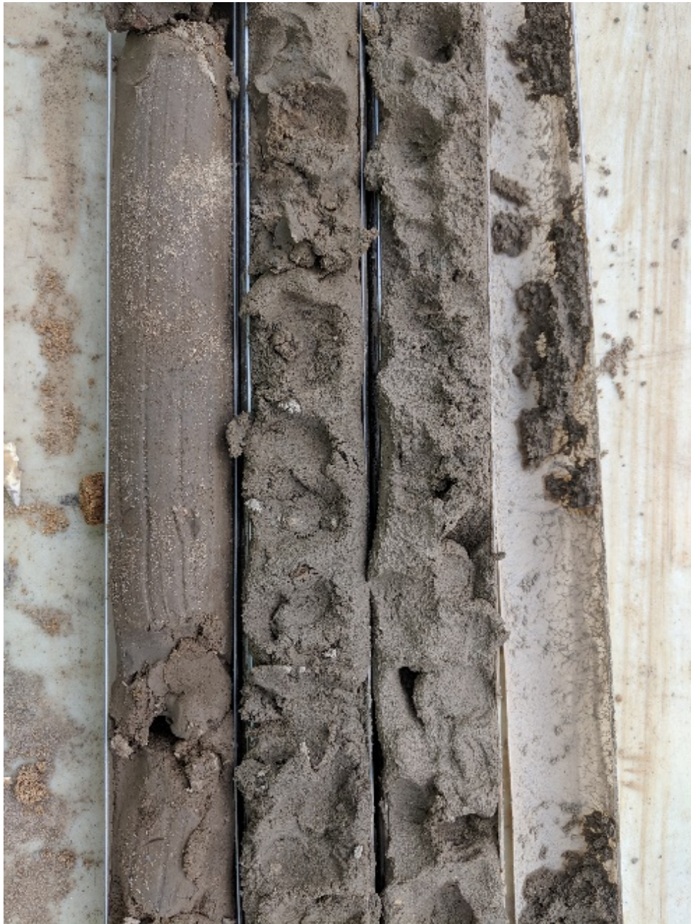
Photograph 2: Slurry wall material core (09-03-2019)
