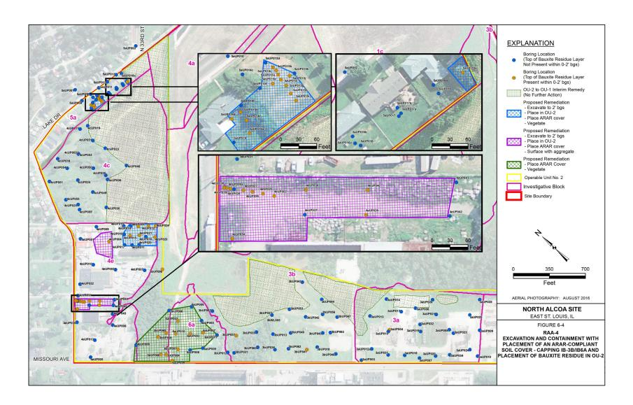
Figure 13: RAA-5 Proposed Excavation/Consolidation/Capping
