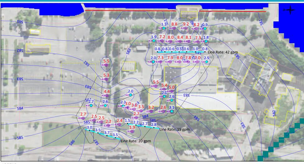
582— Simulated groundwater elevation contour, Model Layer 1 (ft amsl)
