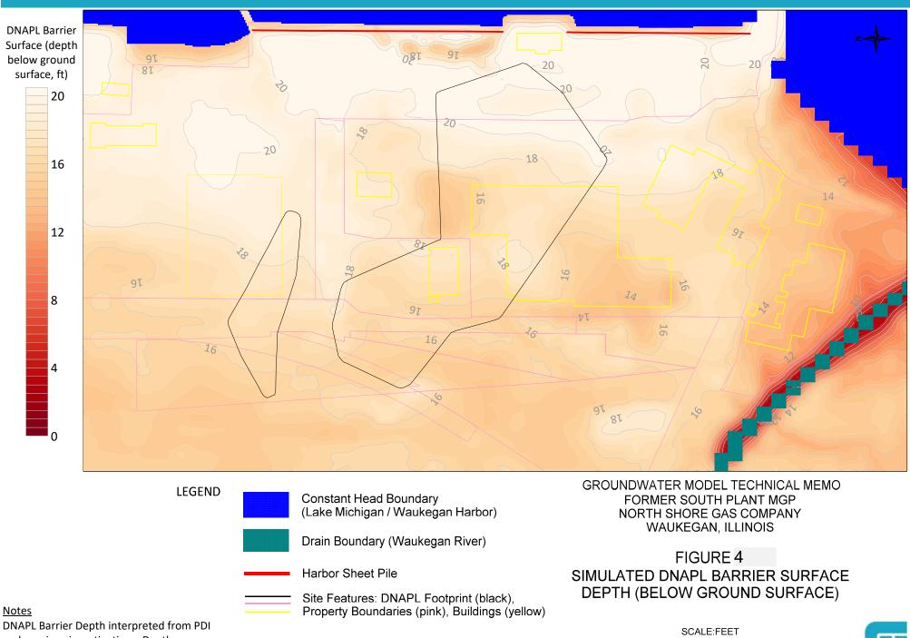
and previous investigations. Depths displayed on map are equivalent to the bottom elevation of Model Layer 2.
