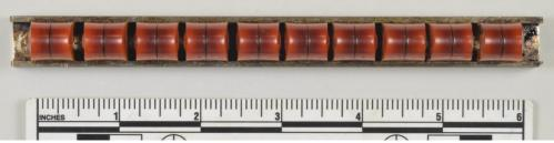
**Figure 3.** Post-test appearance of stressed HDPE test specimens. No cracking was observed on the test specimens. The reason for red discoloration in the stressed area, as opposed to the yellow discoloration of the flat panels, is not known. (The same lot of HDPE was used to prepare all test specimens.)
