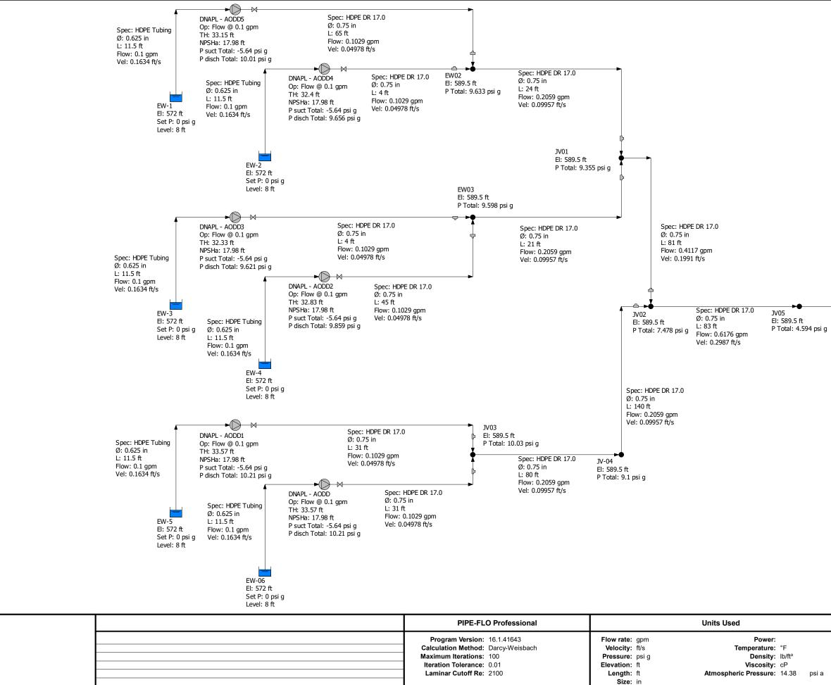
Spec: HDPE DR 17.0 Ø: 0.75 in L: 20 ft Flow: 0.6176 gpm Vel: 0.2987 ft/s Pressure Boundary 1 El: 598 ft Set P Total: 0 psi g
