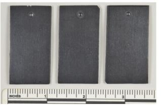
Pre-Test, Back Figure 6. PVDF test specimens
