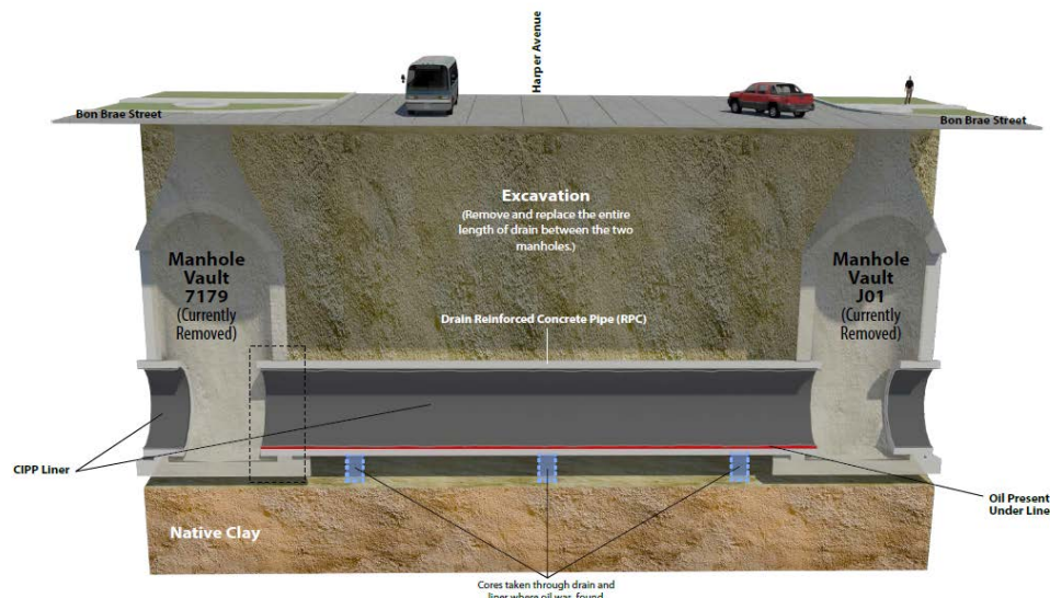
Cross section of pipe beneath Harper Avenue and vaulted manholes
