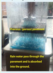
of the lot will be paved with asphalt and will slope toward the perimeter of the lot that will have pervious (porous) pavers. pavers give the appearance of a hard surface however they allow water to pass through them and absorb into the ground. This allows for treatment of the water before it enters the lake. The picture below and the pic-
