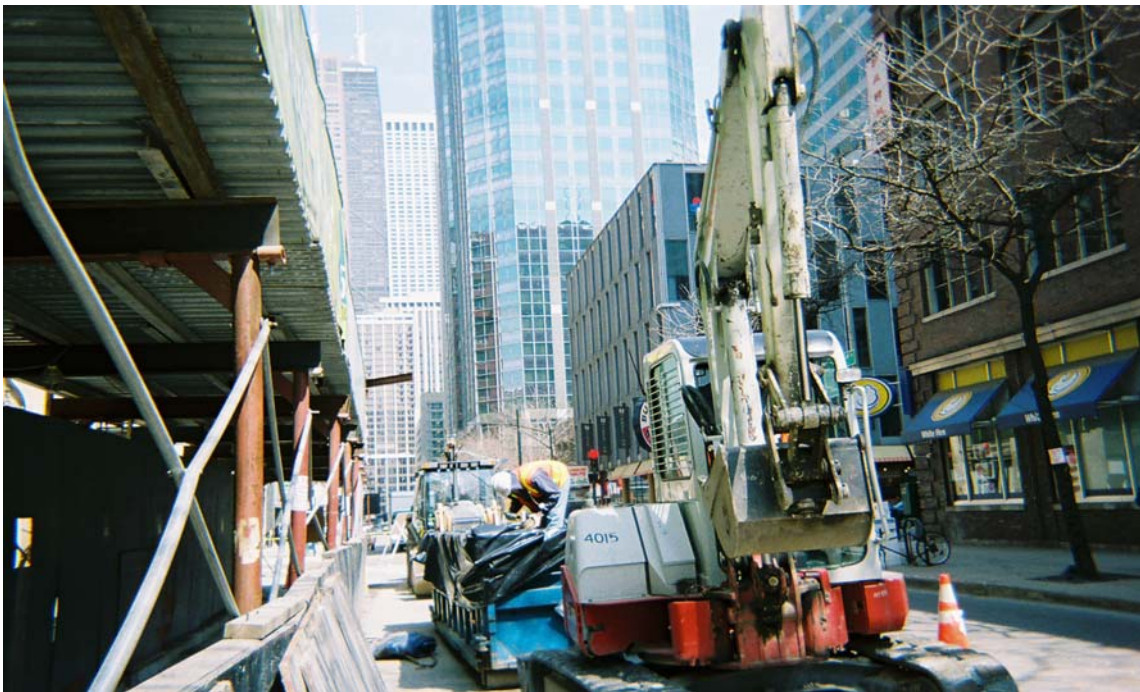
Photo 12: Taken south to north. Shows composite sampling of soil in roll-off boxes using hand auger. Hand auger samples from four locations homogenized in collection tray.
