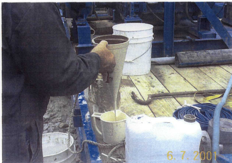
Photo 3. Field QA/QC testing of bentonite-water mixture (slurry).
