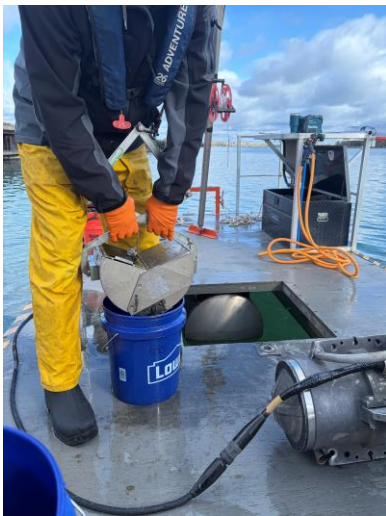
Surface sediment collection via a Ponar dredge sampler
