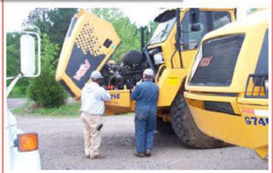
CHECKING EQUIPMENT FLUID LEVELS
