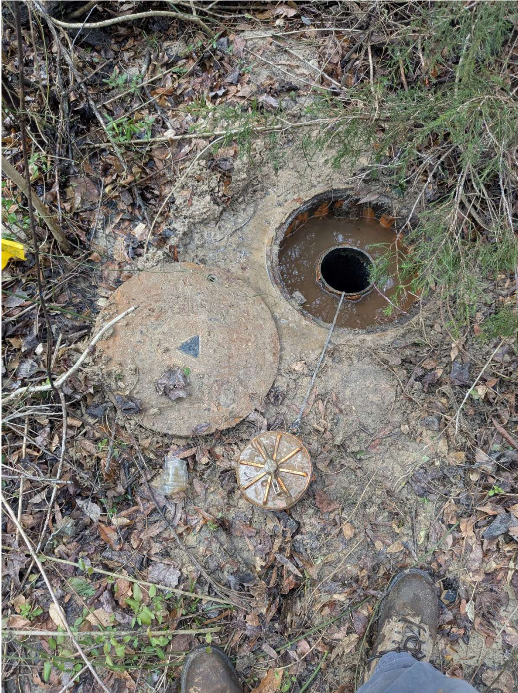
FIGURE C8: MW-2 inner casing was cleared and pumped before sampling
