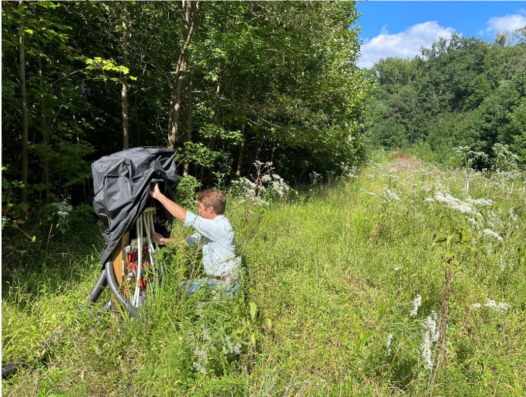
PHOTOGRAPH 04: Solar panels to heat water for circulation through selected upgradient trench pits (See Figure 1). There were no signs of damage or tampering on this system at time of inspection. Vegetation in clearing will require clearing.
