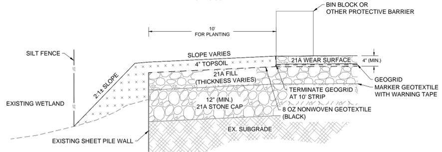
**10' PHYTOPUMPING STRIP (AREA A-2) SECTION WITH ADDITIONAL DRAINAGE GRADING - ABOVE SHEET PILE WALL CONDITION**
