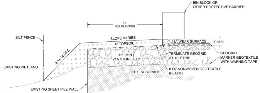
**10' PHYTOPUMPING STRIP (AREA A-1) SECTION - ABOVE SHEET PILE WALL CONDITION**
