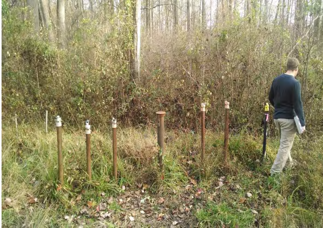
PHOTOGRAPH 05: Transect Wells running perpendicular to the biowall. The transect well second to the right is missing a lock.
