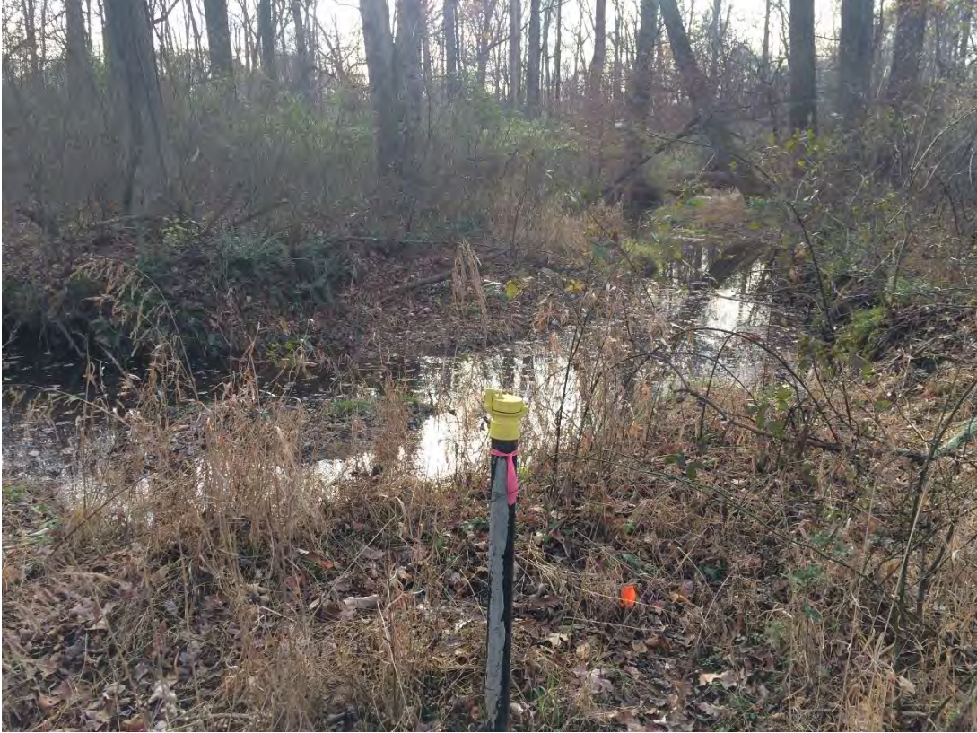
PHOTOGRAPH 07: MW10 near Beaver Dam Creek tributary. MW10 is missing a lock
