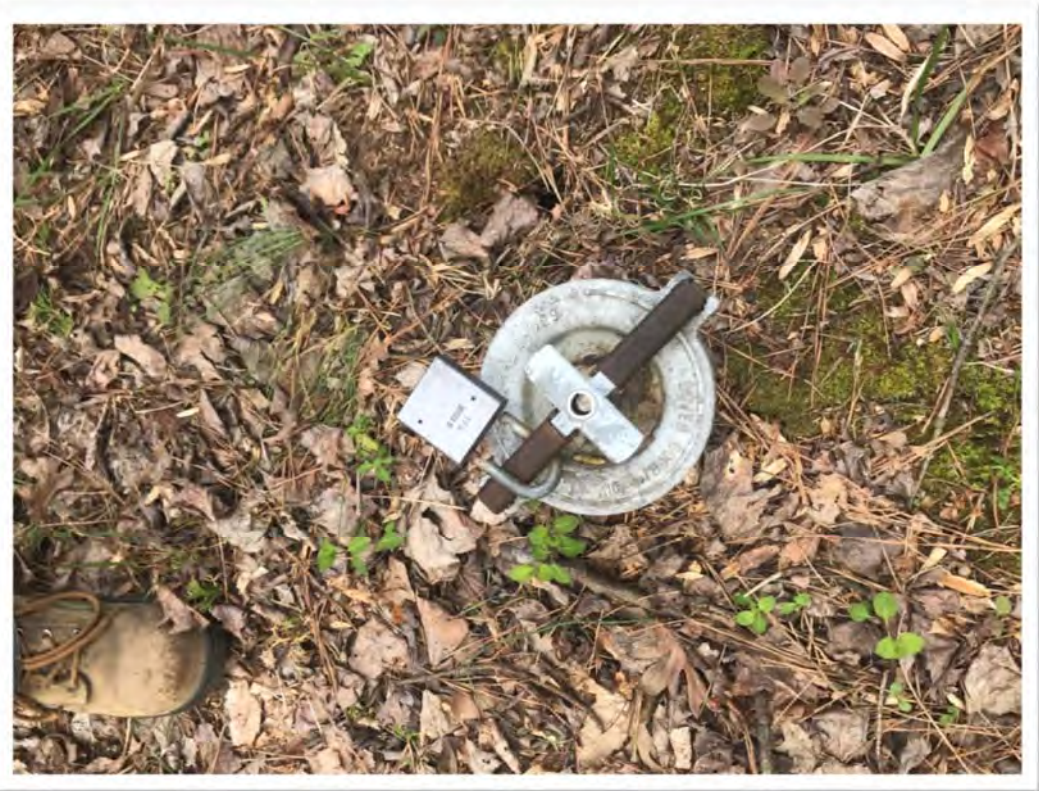
Photo: 017 Date: 04/23/18 Description: At monitoring well, MW-7S. Well cap not locked. Photographer: [REDACTED]
