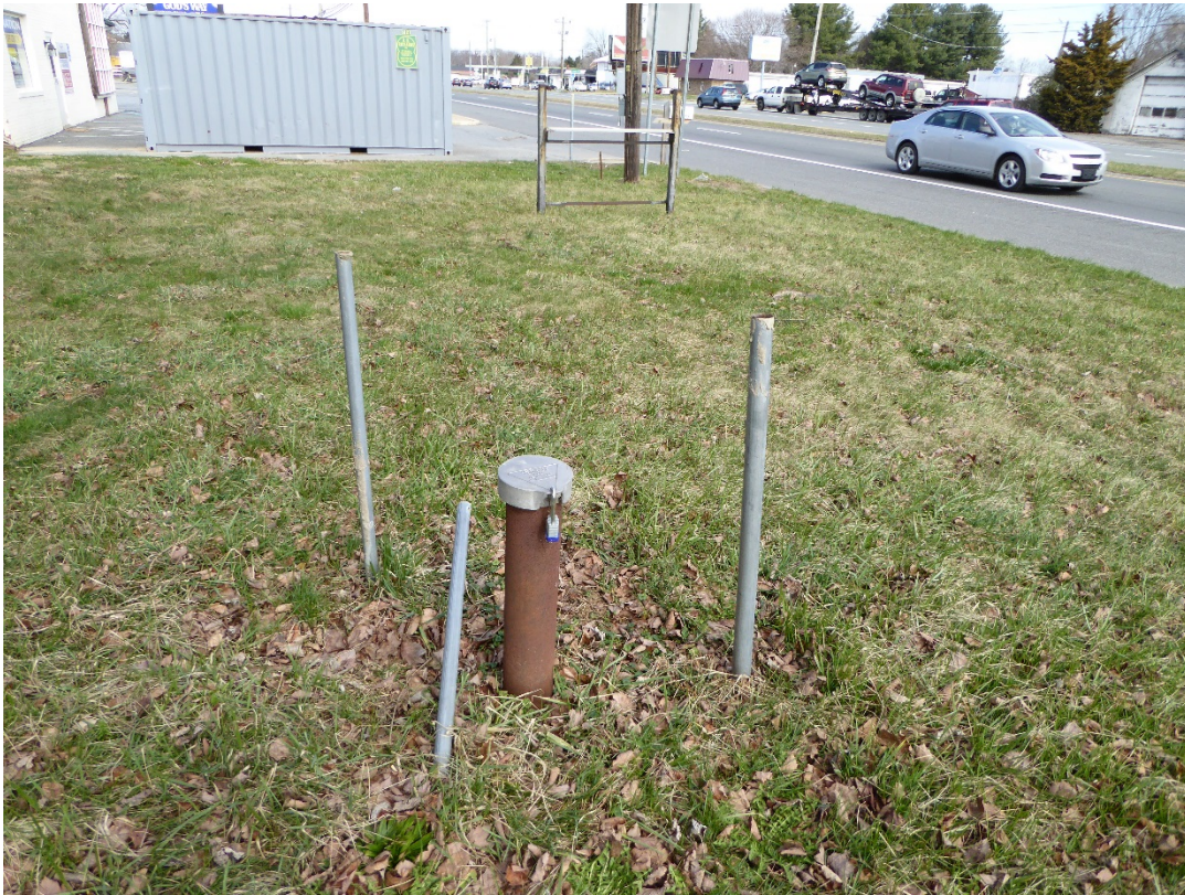
Monitoring well on former facility property
