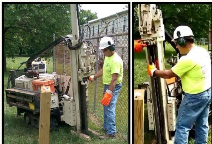
Above: An EPA contractor is shown performing a soil vapor assessment using a Geoprobe Drill Rig.
