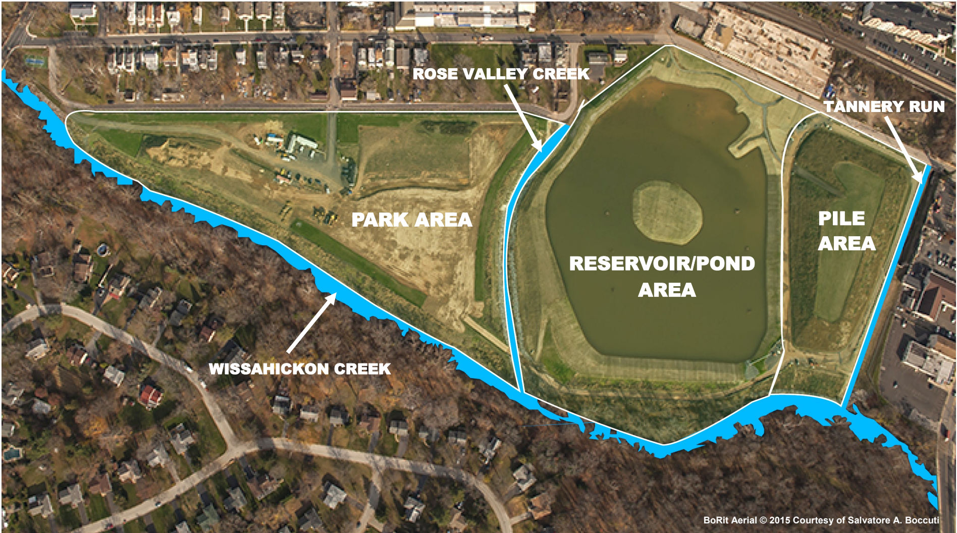
Aerial view of site, taken in November 2015, shows work in progress on the park parcel and work completed on the pile parcel and the former reservoir now called the pond. Improvements made to the pond include a 1/2-acre island for nesting migratory birds and a viewing area and trails along Maple Avenue.
