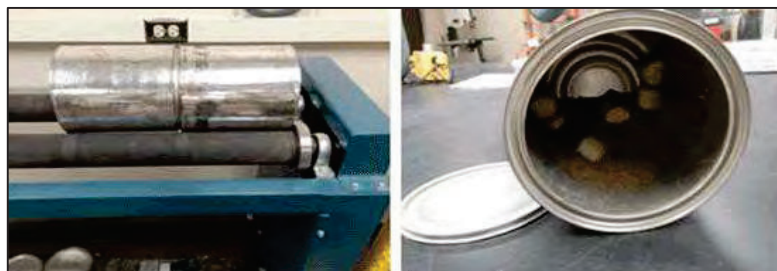
Figure K-5. Ball mill with ceramic cylinders used for moderate crushing of large soil volumes. Ball mills are less able to crush soil to a consistent particle size.
