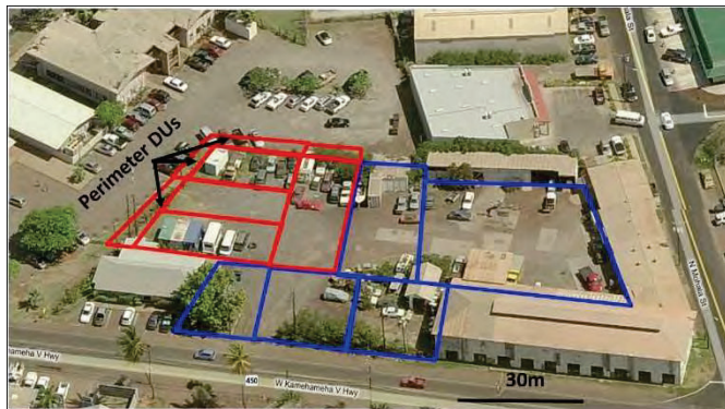
Figure C-2. Designation of Source Area (red) and Exposure Area (blue) DUs at a former electrical power plant to determine the magnitude and extent of PCB-contaminated soil. Former transformer storage and repair operations located in upper left area of the property.
