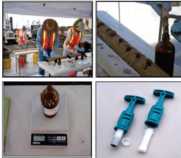
Figure 3-18. Preparation of an MI sample to be tested for VOCs by placing sample increments
