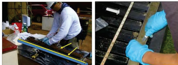
Figure G-7. Subsampling of Core Increments for Preparation of a Bulk Multi Increment Sample.
