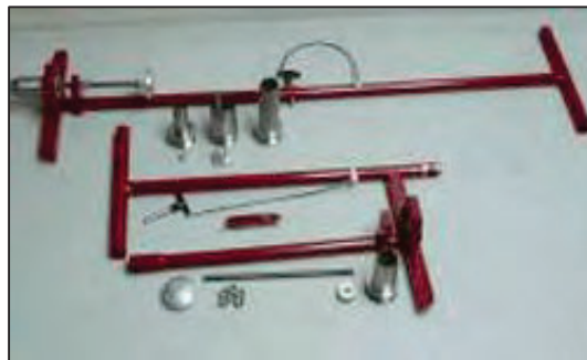
Figure F-8. Foot-operated core sampling device developed by the US Army Corps of Engineers (USACE 2007).
