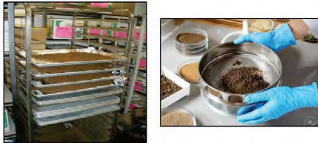
Figure-K-1. Air drying and sieving of samples.
