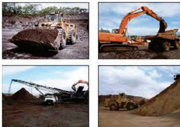
Figure H-3. Examples of opportunities to collect increments and Multi Increment samples during stockpile formation or movement of soil.
