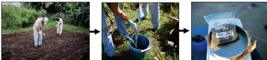
Figure F-7. Collection of increments with a sampling tube.
