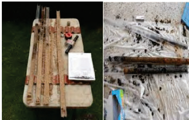
Figure G-5. Continuous Cores Collected using a Push Rig
