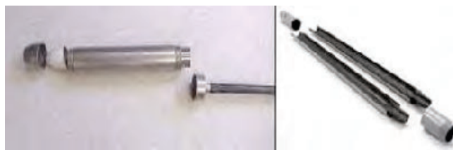
Figure G-4. Split spoon sampler.
