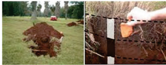
Figure C-10. Backhoe potholes used to collect increments from three subsurface layers designated for DUs at a former golf course (see Figure C-9).
