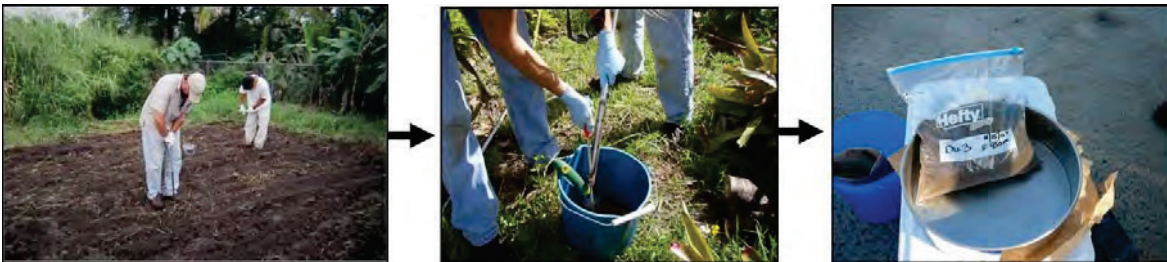
Figure 3-10. Collection of a sample increment and progressive combination of increments to preparation of a single MI sample for the targeted DU.
