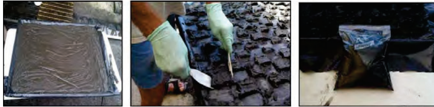
Figure J-8. Field subsampling of a sediment Multi Increment bulk sample.
