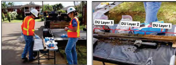
Figure G-6. Identification of targeted DU Layers in cores.
