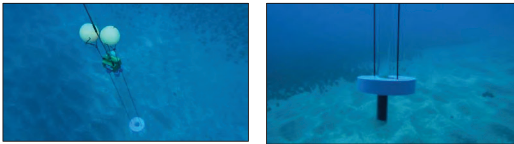
Figure J-6. Submersible platform used to collect sediment increment cores within a targeted DU (manufactured by Specialty Devices Inc.).
