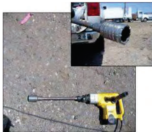
Figure F-17. Tunnel bit uses to cut through asphalt or concrete and access soil (Dewalt 7 cm diameter bit shown).
