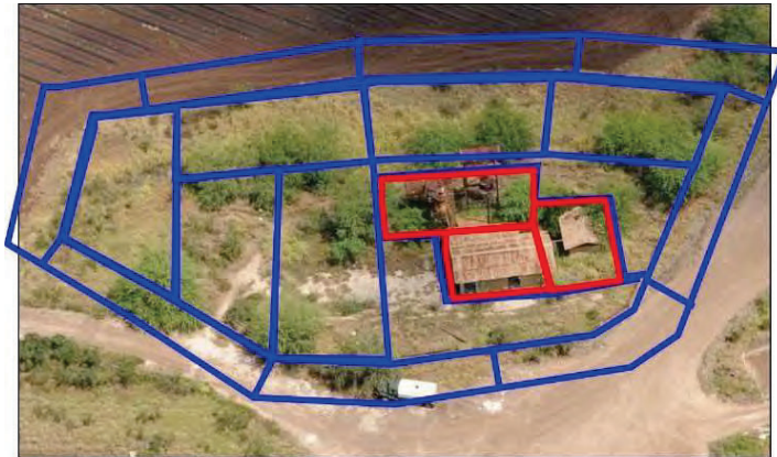
Figure C-3. Example Source Area DUs (red), Exposure Area DUs (blue), and Boundary Area DUs (blue, outside ring) designated for investigation of a former pesticide mixing and storage area.
