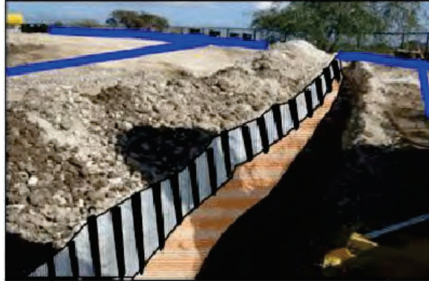
Figure G-10. Use of shallow trenches to collect samples from exposed DU Layers. Surface DU boundaries noted in blue. Surface sample (0-15 cm) collected prior to excavation of trenches. Increments for subsurface DU layers collected across the full vertical thickness of the exposed targeted horizon to prepare a bulk sample (layers depicted).
