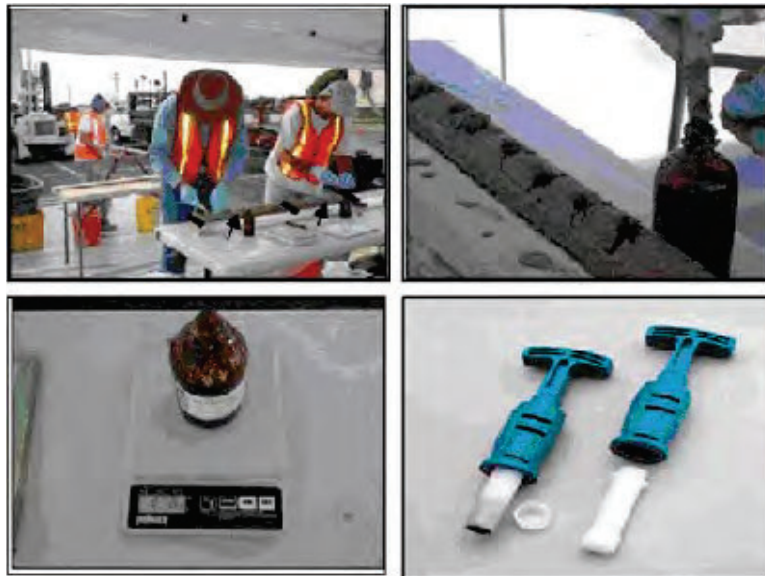
Figure I-1. Subsampling DU Layer increments from borehole cores with methanol preservation.
