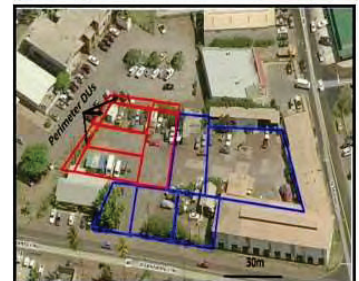
DUs are designated to answer specific risk or remediation questions. The entire property is often tested.
