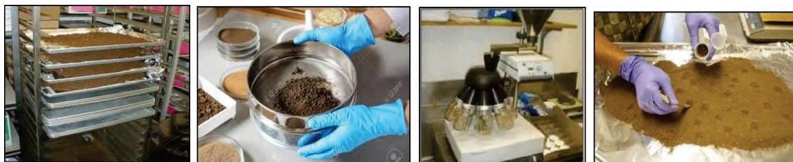
Figure 3-21. Collection of an analytical subsample from a MI sample after air drying and sieving.
