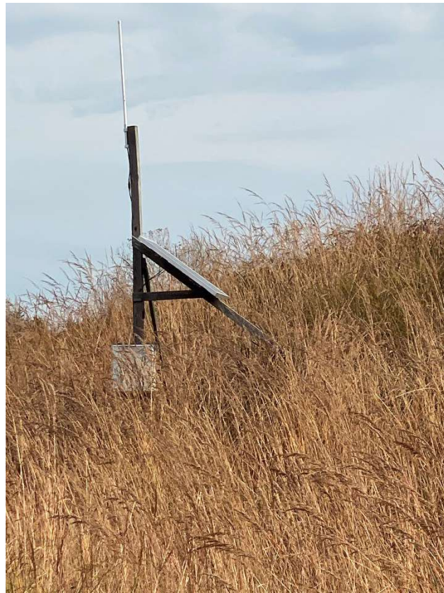
Solar-powered receiver receives monitoring well data from across the river
