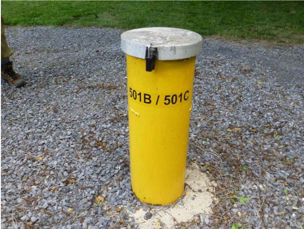
Locked monitoring well on the west side of the river
