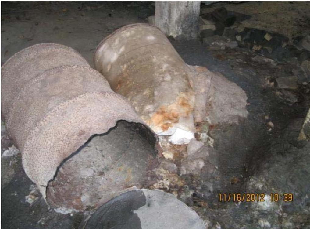
View of the deteriorated drum containing asbestos pipe insulation at the Area C basement.
