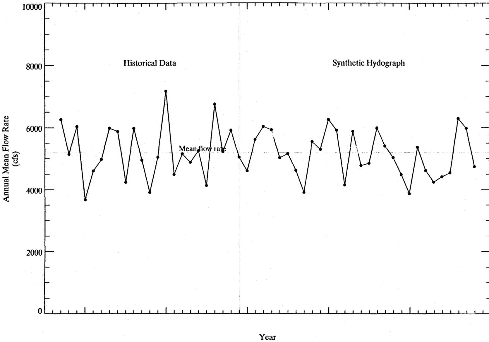
Figure 3-4. Annual mean flow rate at Fort Edward (1975 to 2028). The extended synthetic hydrograph begins in 1999.
