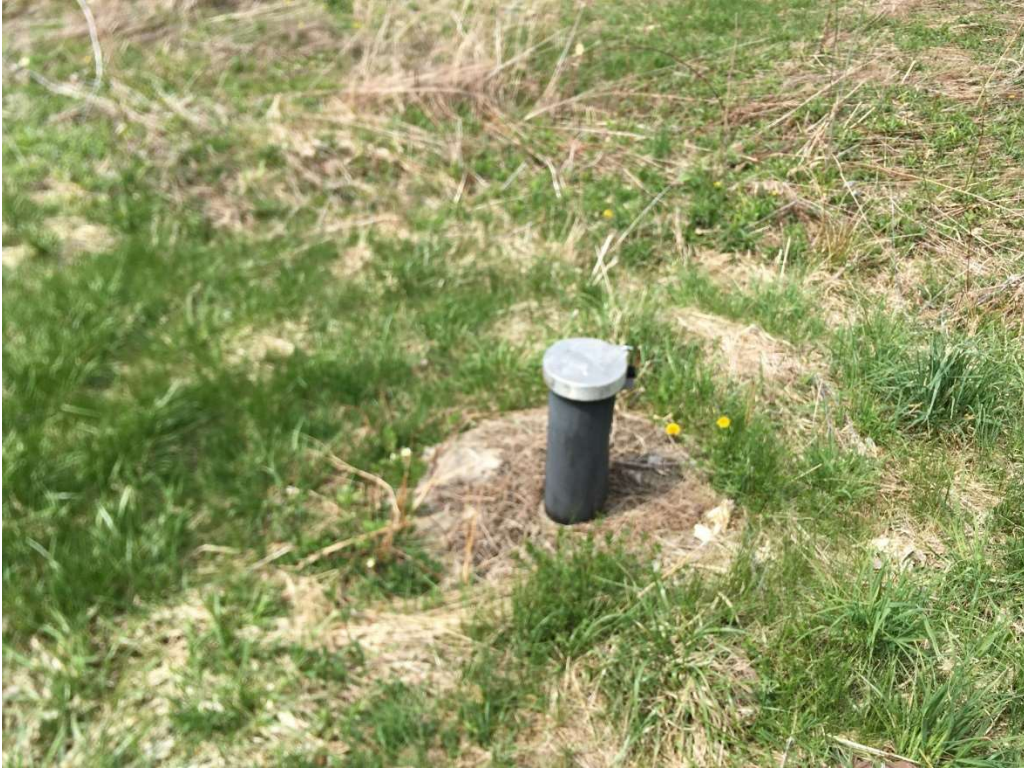
Photo of Perimeter Monitoring Well – West Side
