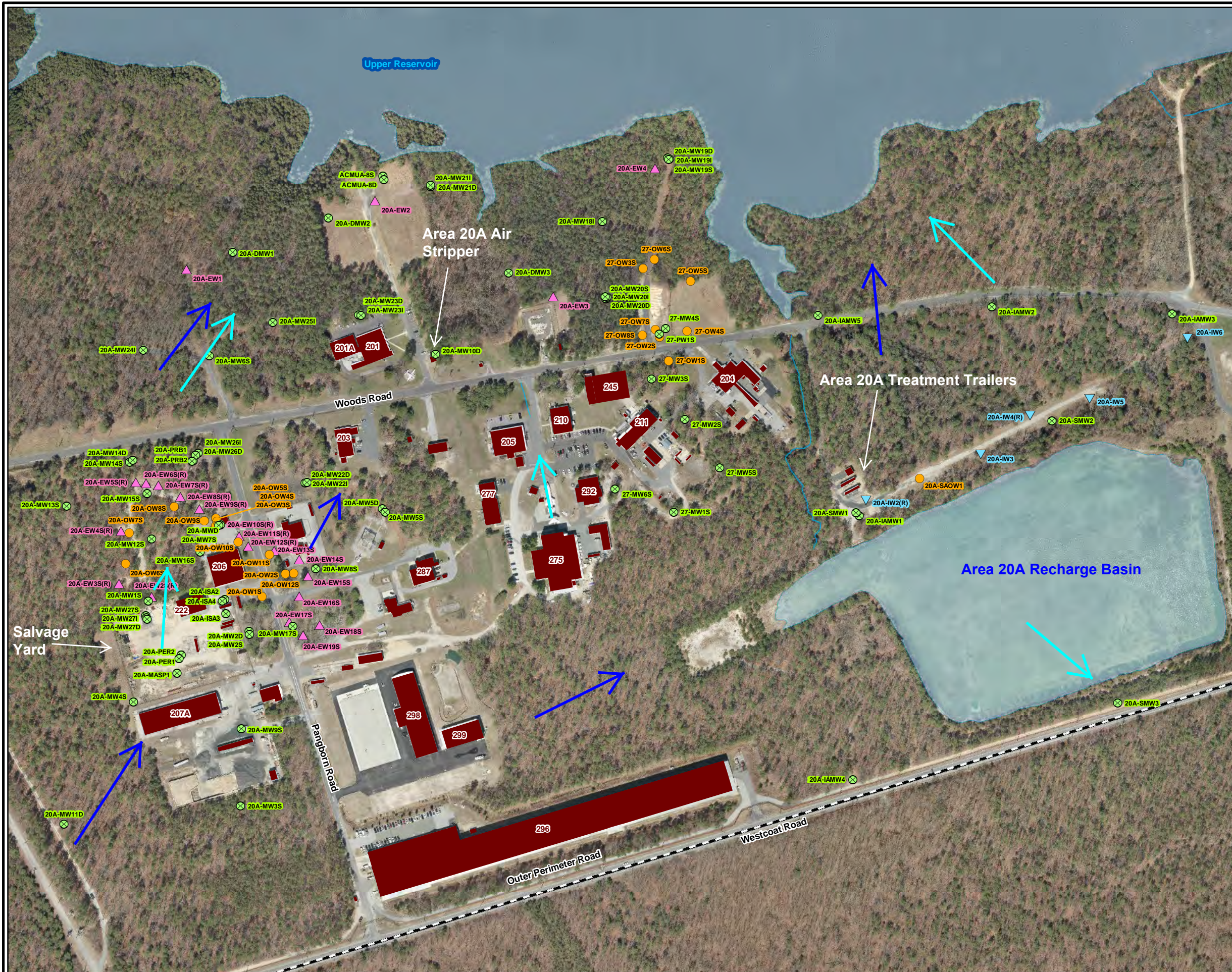
Figure 5 Area 20A Extraction and Monitoring Well Locations and Groundwater Flow Directions
