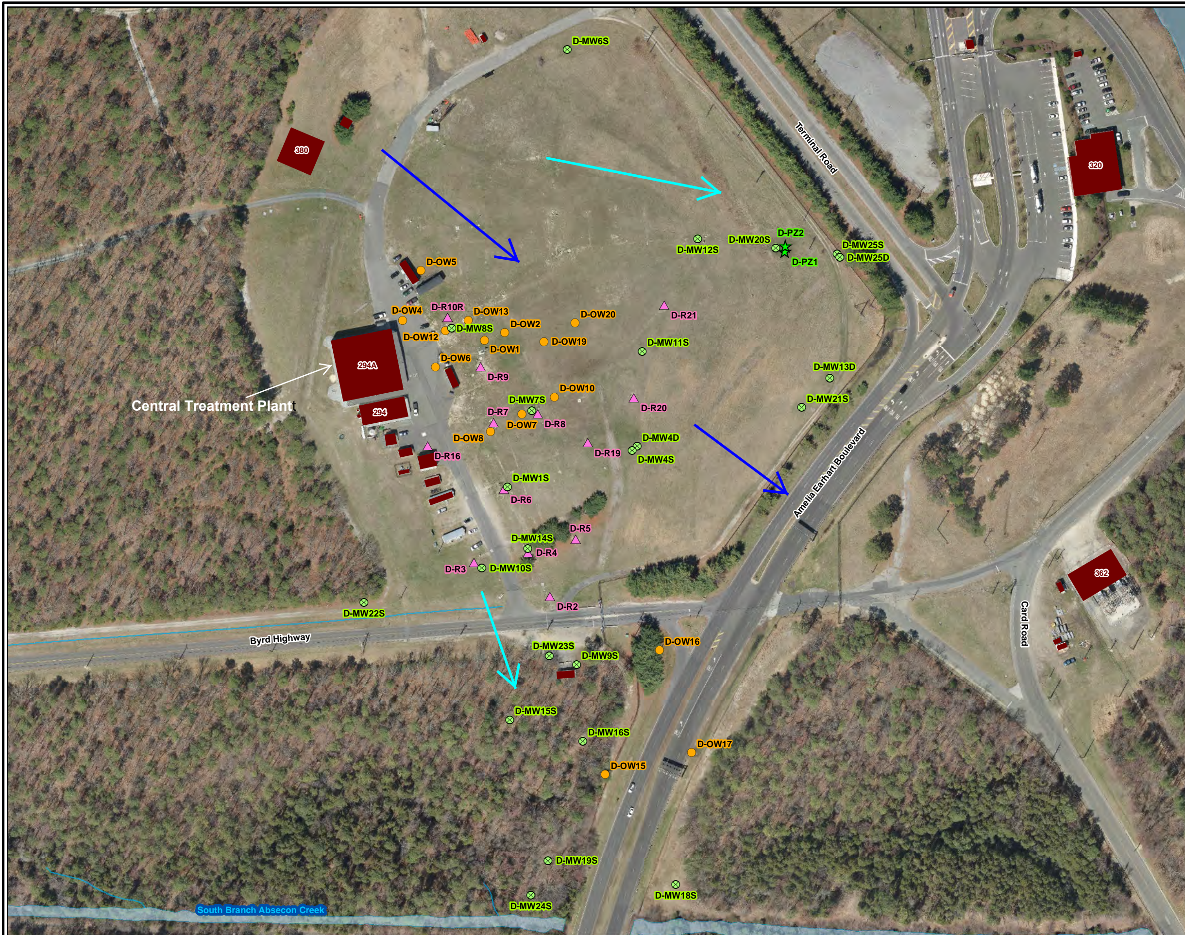
Figure 4 Area D Groundwater Well Locations and Groundwater Flow Directions
