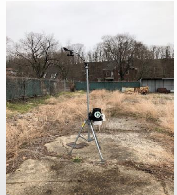
Mobile meteorology sensor
