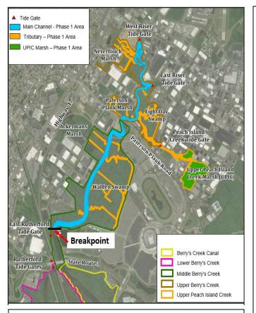
*Breakpoint* is a location in Middle Berry's Creek where changes in the physical system result in a step-wise change of contaminant concentrations upstream and downstream of this point.
