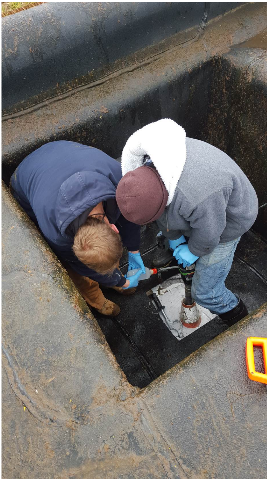
3 – December 16, 2015: Concrete core drilling at Sample Location 6
