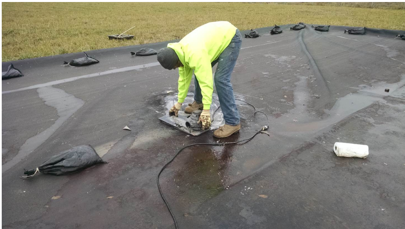
2 – December 16, 2015: Vacuum testing HDPE liner repair at Sample Location 3
