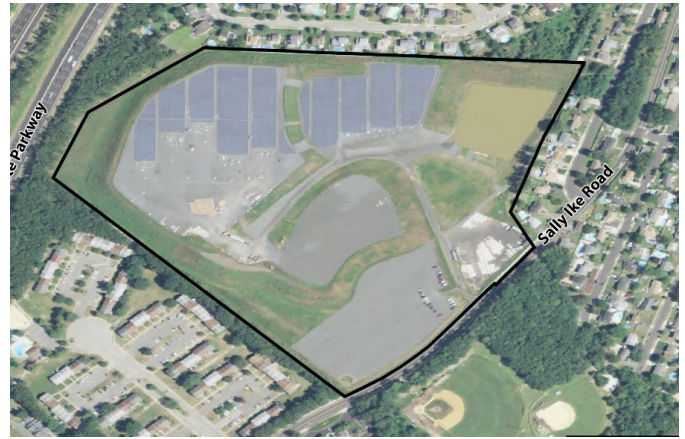
2013 aerial photo of Brick Township Landfill during redevelopment, with about half of the solar panels installed.
