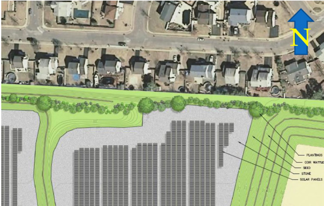
The project's design engineers beautified the cap by planting trees and shrubs near homes.
