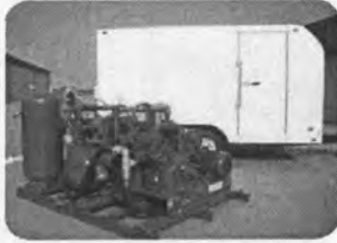
200 cubic meter / hr pilot unit blower, compressor and after cooler
