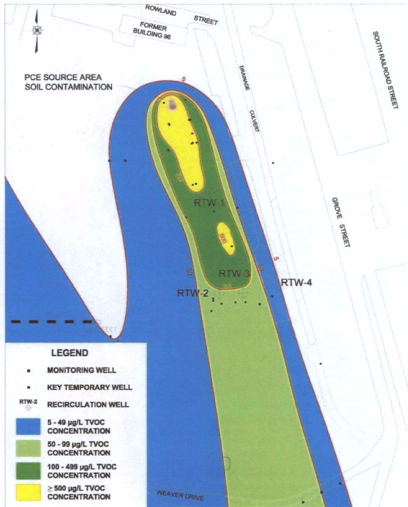
Figure 1. Location of Building 96 Groundwater Plume, Treatment Wells, and Soil Contamination Source Area
