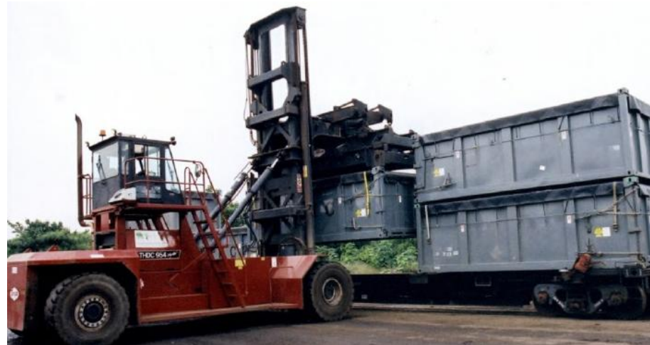
Loading container to rail
