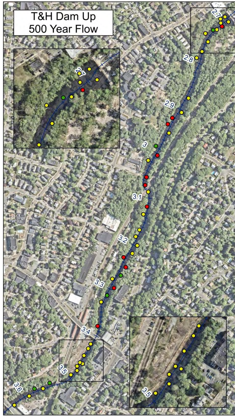
Figure 8. Sediment Stability Results for 500-year Flood Conditions
