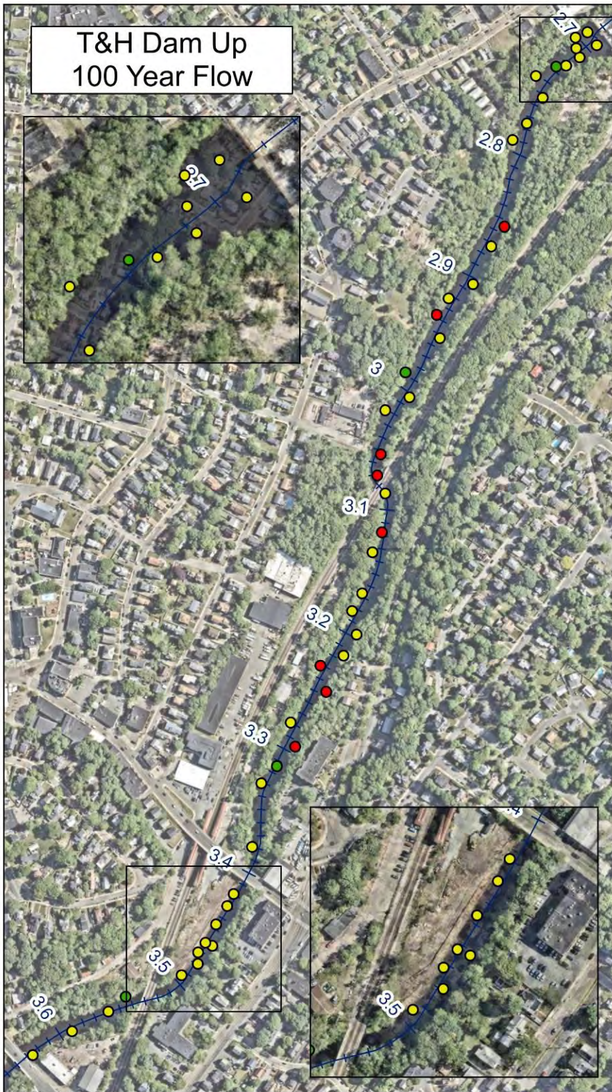
Figure 7. Sediment Stability Results for 100-year Flood Conditions
