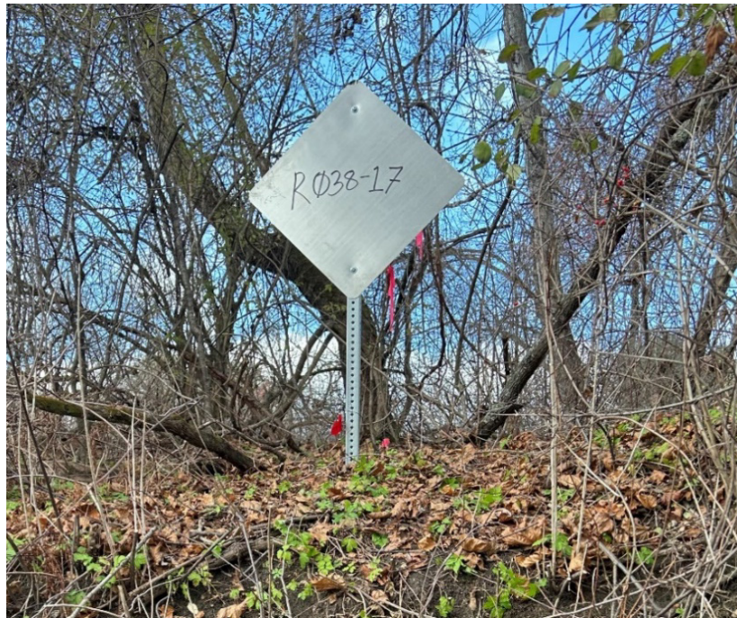
Figure 5. LiDAR Control Monument
