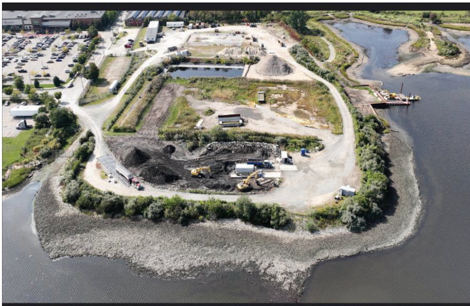
Figure 16: Pilot CDF Shore- line Cap (the rocky surface seaward of the Sawyer Street facility). Aerial view looking west at low tide. Photo: Ed Pepin
