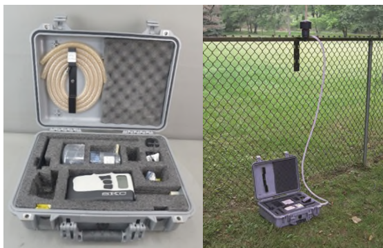
Figure D-4 Battery-powered air sampling equipment for PCBs, courtesy of SKC Inc.
