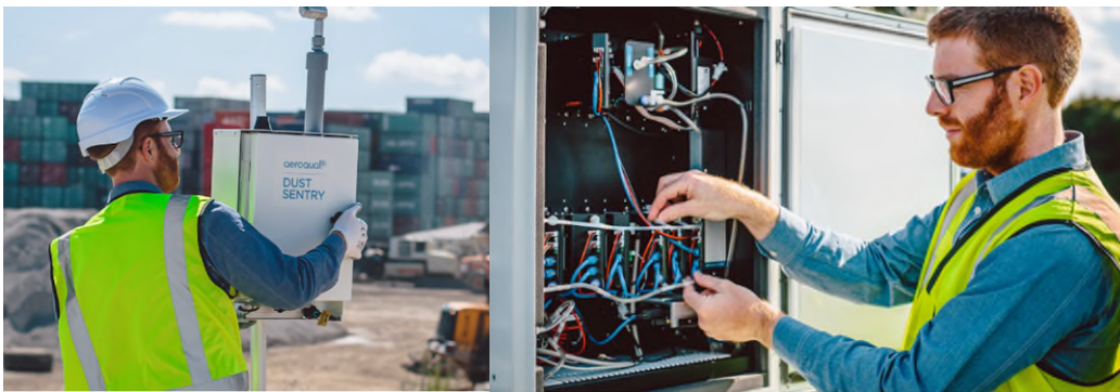
Figure D-2 Deployable particulate air monitoring station, photos courtesy of Aeroqual, Inc.
