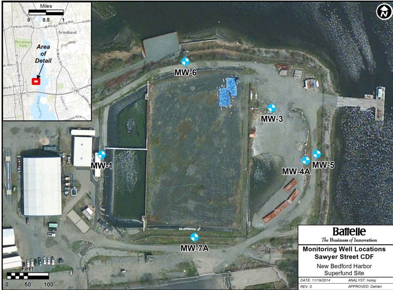
Figure 1. Sawyer Street CDF Monitoring Well Locations
