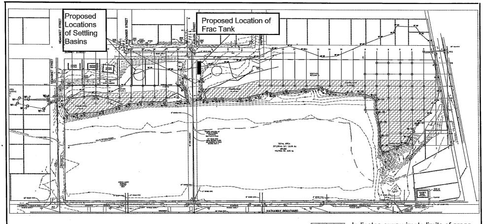
Indicates approximate limits of areas to be cleared and PCB-impacted sediments to be removed (PCB concentrations > 1 ppm)
