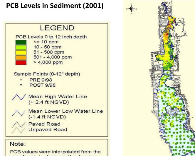
PCB values were interpolated from the sample points shown on the drawing. PCB values at any location were assumed to be equal to the PCB value of the closest sample point.
