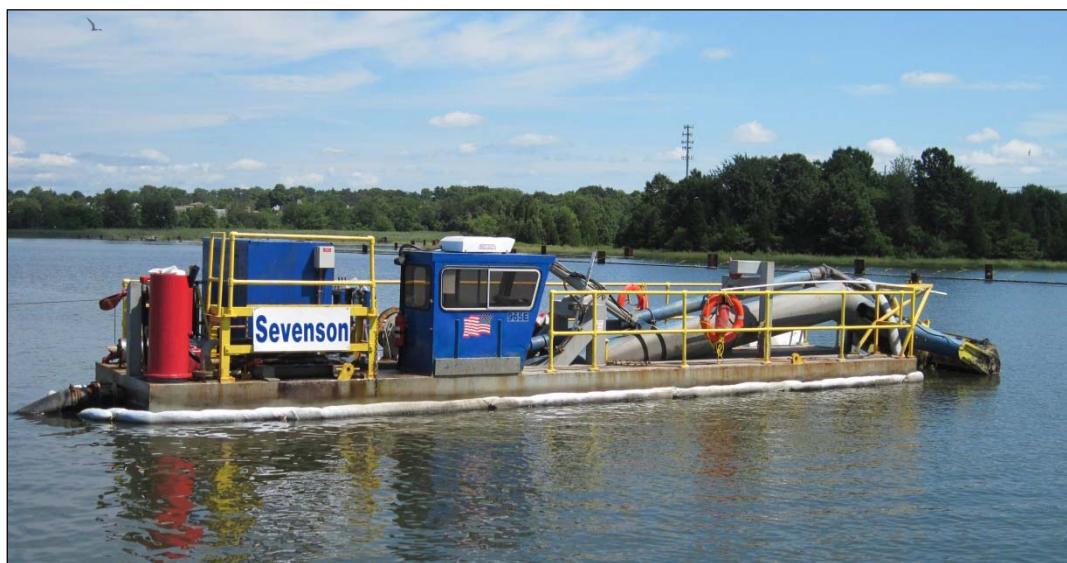
Figure 7. Mud Cat TM hydraulic dredge
