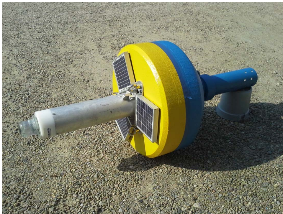
Figure 6. Remote Monitoring Telemetry System Buoy.
