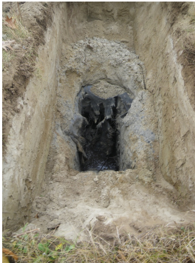
Figure B-4. Test Pit at Transect 3, 0 – 10 Feet, Showing Cap, Geotextile Barrier, Grading Sand and Soil at the Water Table
