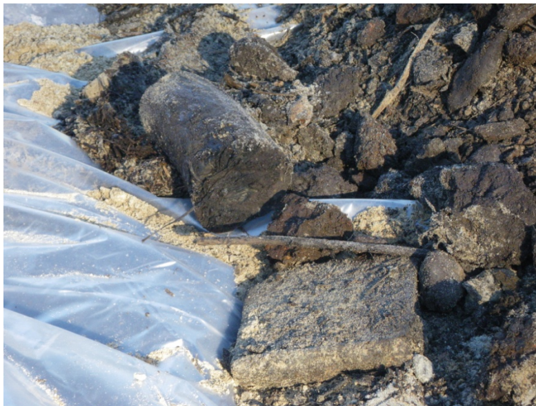
Figure B-5. Buried Construction Debris from Test Pit at Transect 3, 60 – 70 Feet
