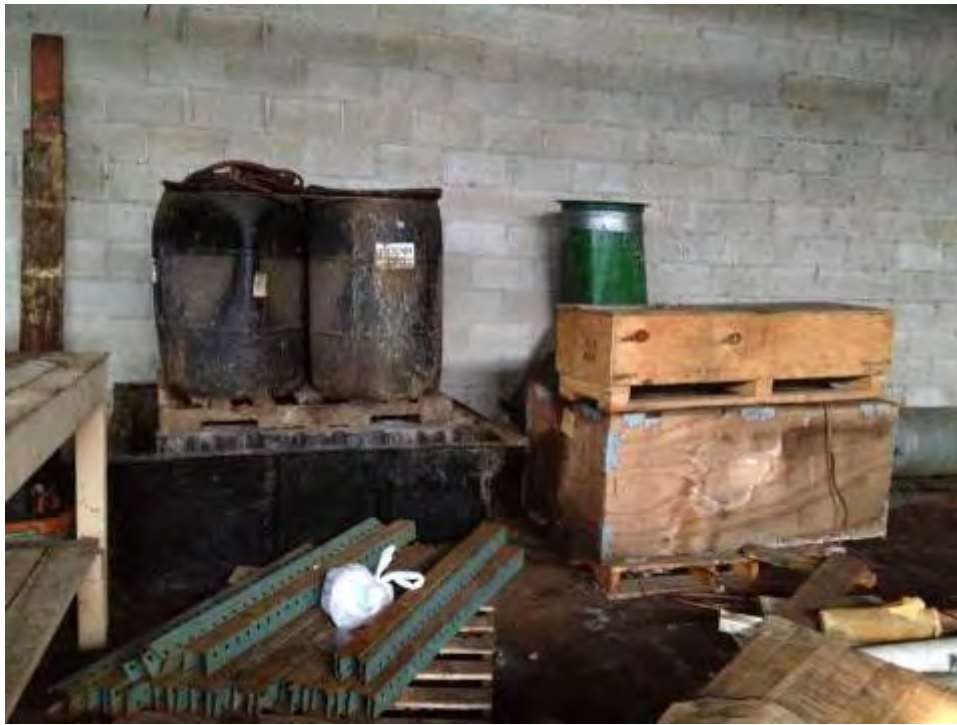
SCENE: View of drums staged on pallets over a secondary containment unit, located west of the Caustic tank.
