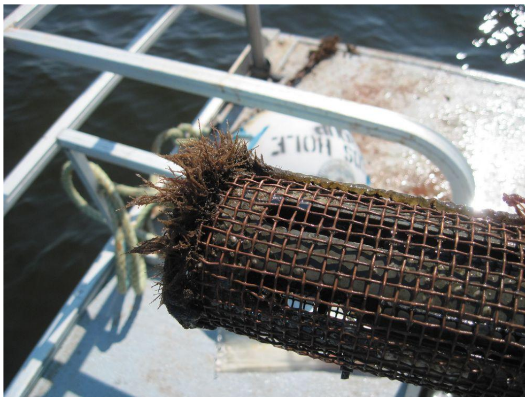
Figure 2. Biofouling (hydroids) on instrument 1000S in September 2012.
