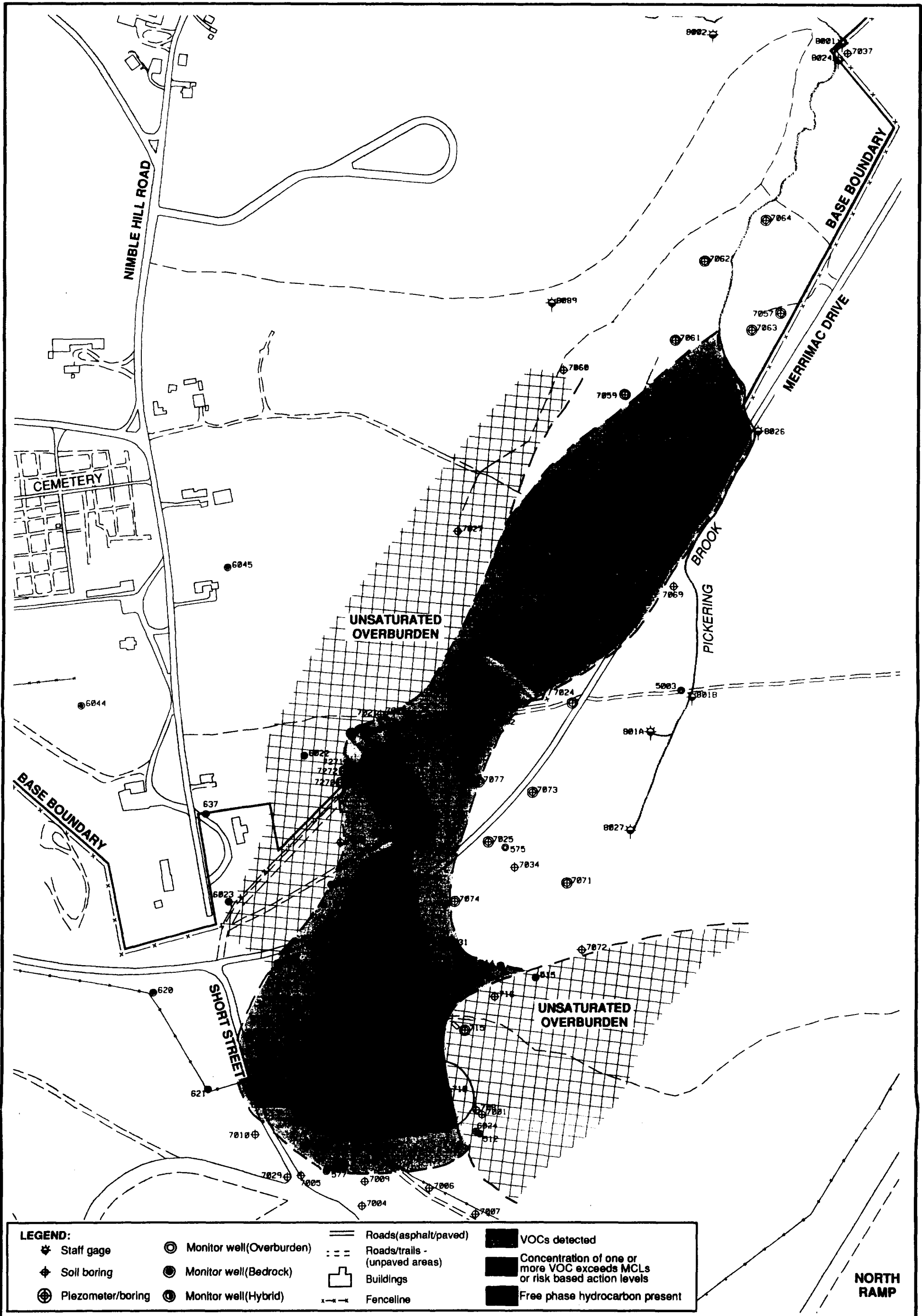
Site 8 (FTDA-2) Stage 3, Record of Decision Pease Air Force Base, New Hampshire FIGURE 9 EXTENT OF TOTAL VOCs IN OVERBURDEN GROUNDWATER
