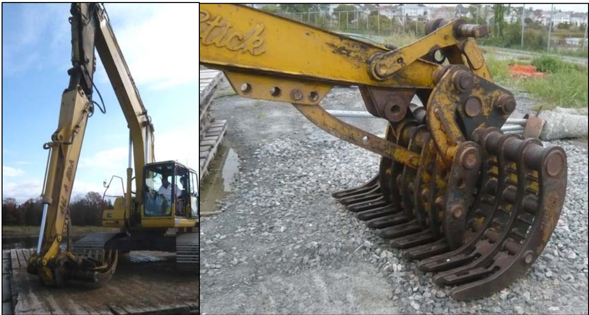
Figure 1-4. NBHSS debris removal machine equipped with "grabber" attachment (photographs by David Robinson).
