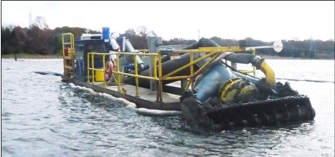
Figure 1-3. NBHSS hazardous sediments dredging barge. Note the horizontal auger-like dredge-head at the barge's bow (photograph by David Robinson).
