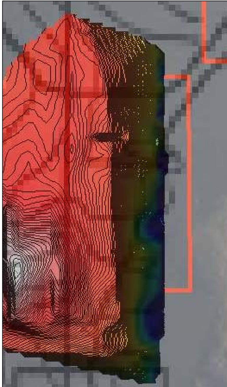
Figure 3-2. Color-coded contour plot of magnetic data recorded during the 2009 geophysical survey of the NBHSS shipwreck study area (image courtesy of CRE).
