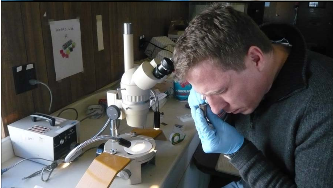
Figure 2-8. Wood samples from a select representative sample of key structural elements of the shipwreck's hull were extracted and subjected to macro- and microscopic analyses in January 2010 by the project archaeologist and archaeological wood specialist, Dr. Brian Jordan. The purpose of this analysis was to identify the wood species used in the vessel's construction, to determine whether the wood was extracted from "old" or "new" growth forests, and to develop hypotheses regarding the general age and origin of the raw materials used in the vessel's construction (photographs by David Robinson).
