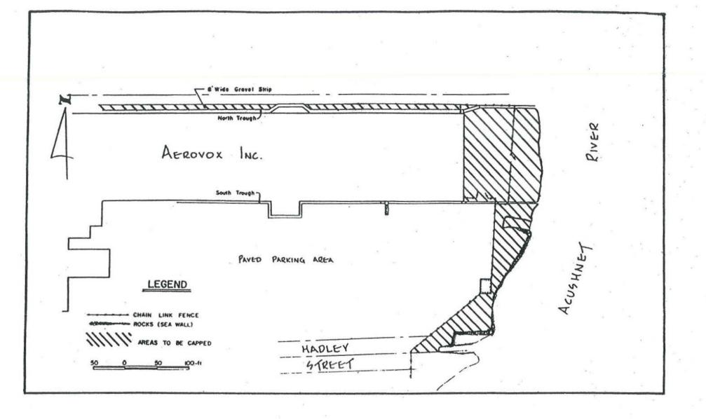
Figure 3 - Area of the Aerovox site covered with the hydraulic asphalt concrete (HAC) cap Vacant Aerovox Plant Supplemental EE/CA, April 2006
