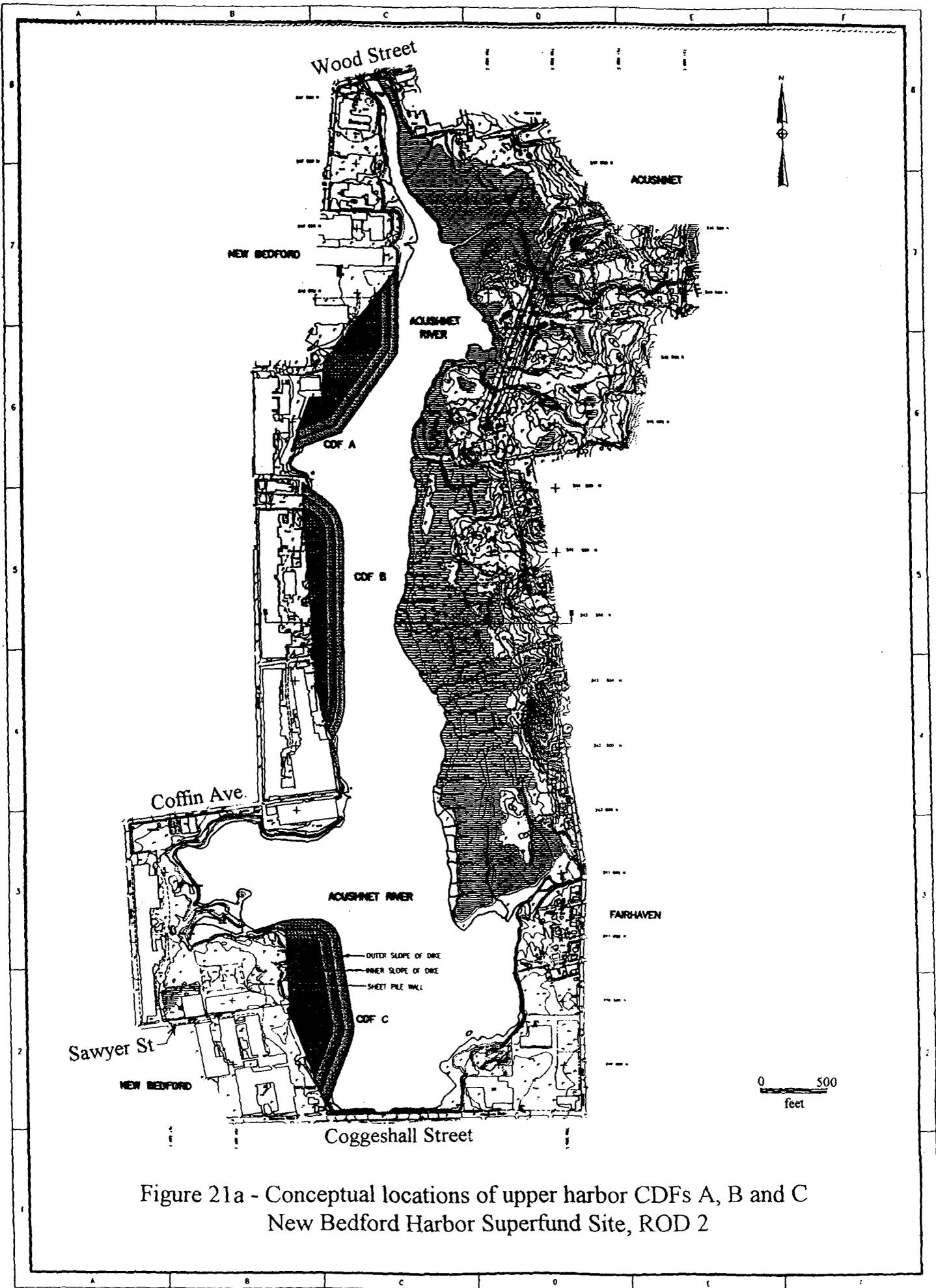
Figure 21a - Conceptual locations of upper harbor CDFs A, B and C
