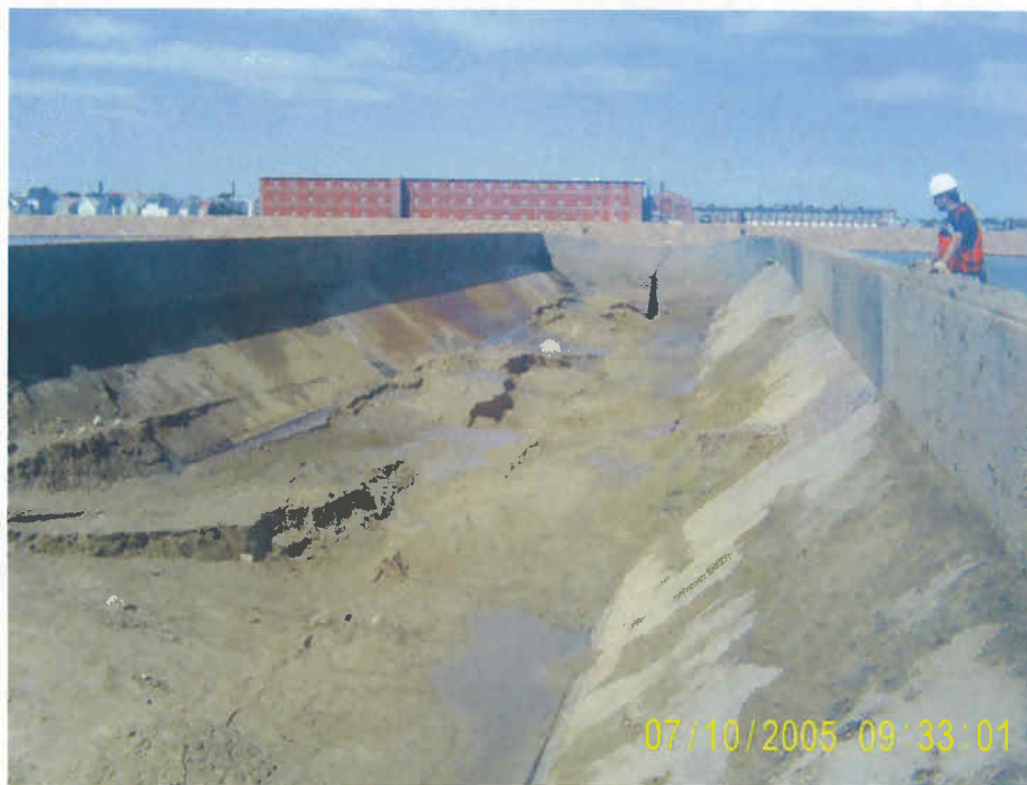
Figure 3: a split-hull scow begins opening to place cap material
