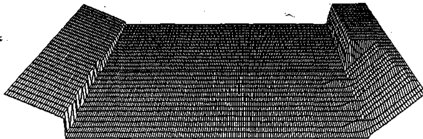
Figure 7—Channel shape after three days of continuous eroding flow.
