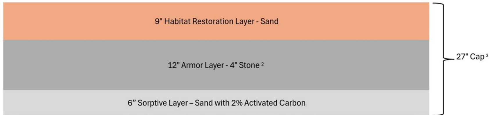
Conceptual Design of Multi-Layer Cap – Excerpt of Figure 16 from EE/CA Report
