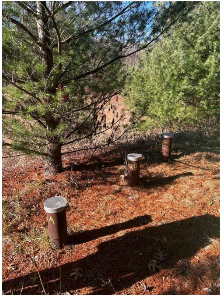
Monitoring wells OSA-13 A, B and C
